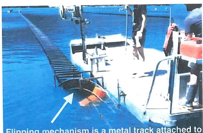
Flipping mechanism is a metal track attached to the side of the boat that turns over the Hexcyl baskets as the boat drives forward. It is not motorized and it is quiet.
