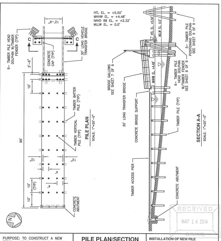
FERRY LANDING, INCLUDING ACCESS PIER, TRANSFER BRIDGE, BRIDGE SUPPORT STRUCTURE, AND BERTHING DOLPHINS.
