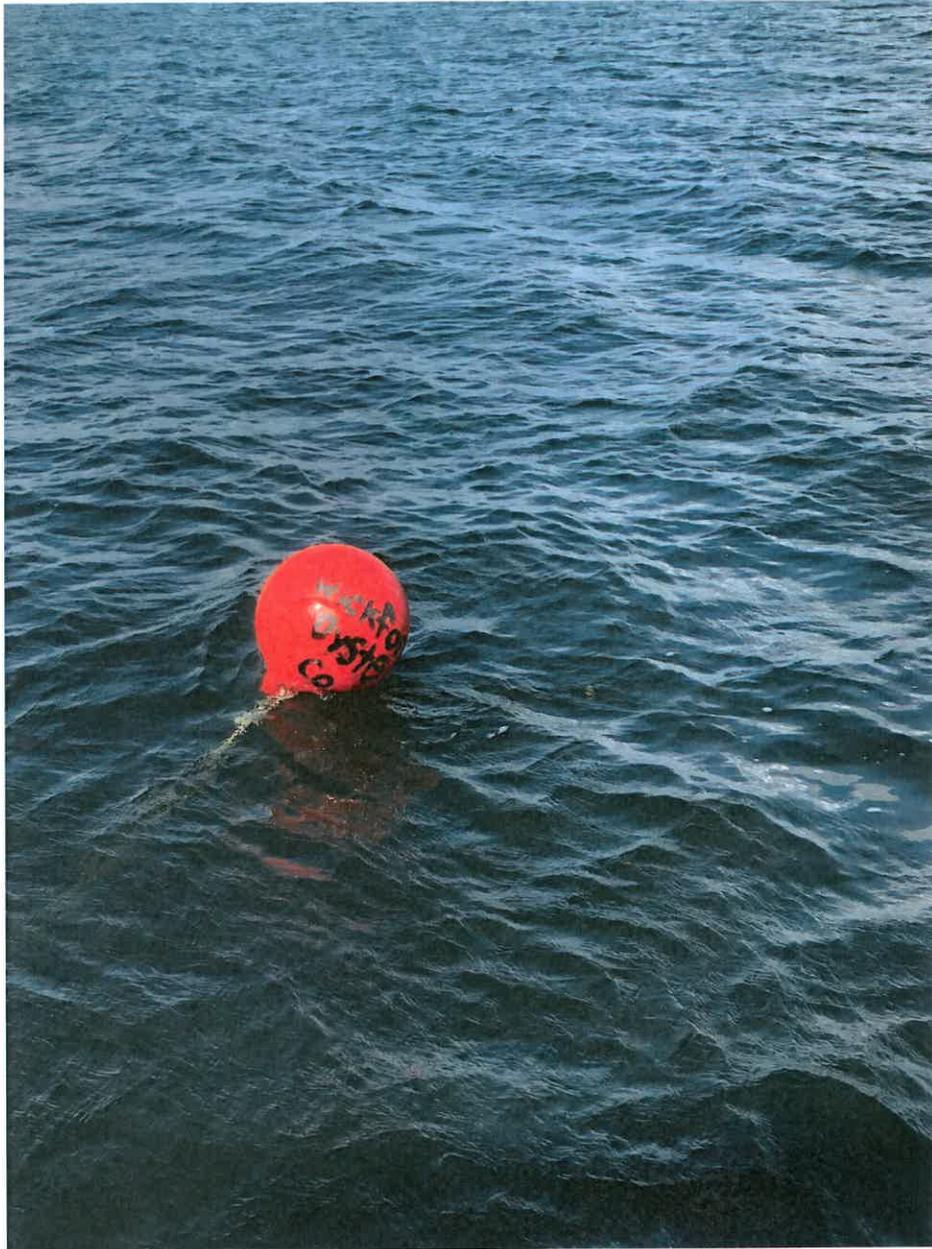
Example of a single Polyball that will mark the location of each mooring attached to the mainlines.
