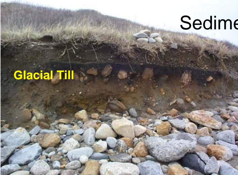
Lower gradient slope less susceptible to erosion until the toe is undermined in a storm
