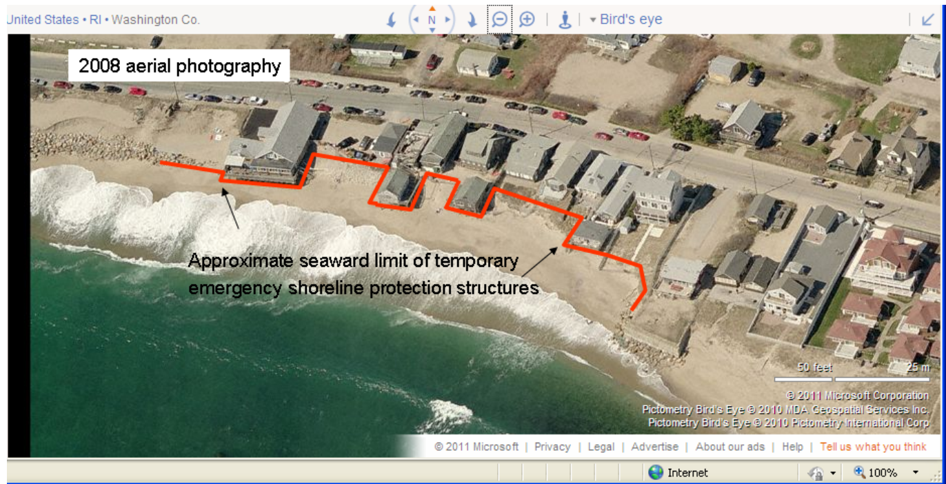
Figure 5. Potential location of temporary wooden bulkhead shoreline protection structures
