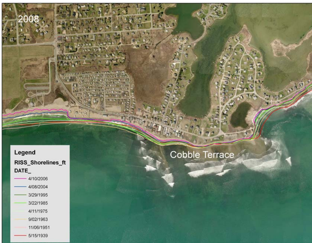
Figure 14. Matunuck Shoreline showing the offshore cobble terrace that dissipates wave energy and helps mitigate erosion along a portion of the Matunuck Headland shoreline. The delineated shorelines indicate which areas change very little over time (lines closer together) and which sections undergo radical change (lines farther apart). The Matunuck Business District has a moderate erosion rate and likely benefits from the offshore cobble terrace which dissipates wave energy.
