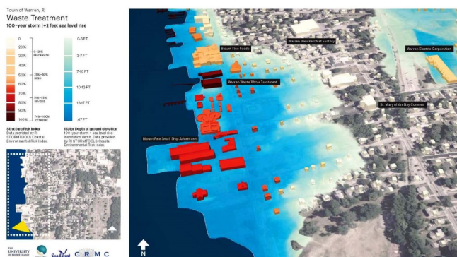
Visualization of the Town of Warren's waste water treatment facility, and its vulnerability under a scenario of 2 feet of sea level rise and a 100-year storm event.
