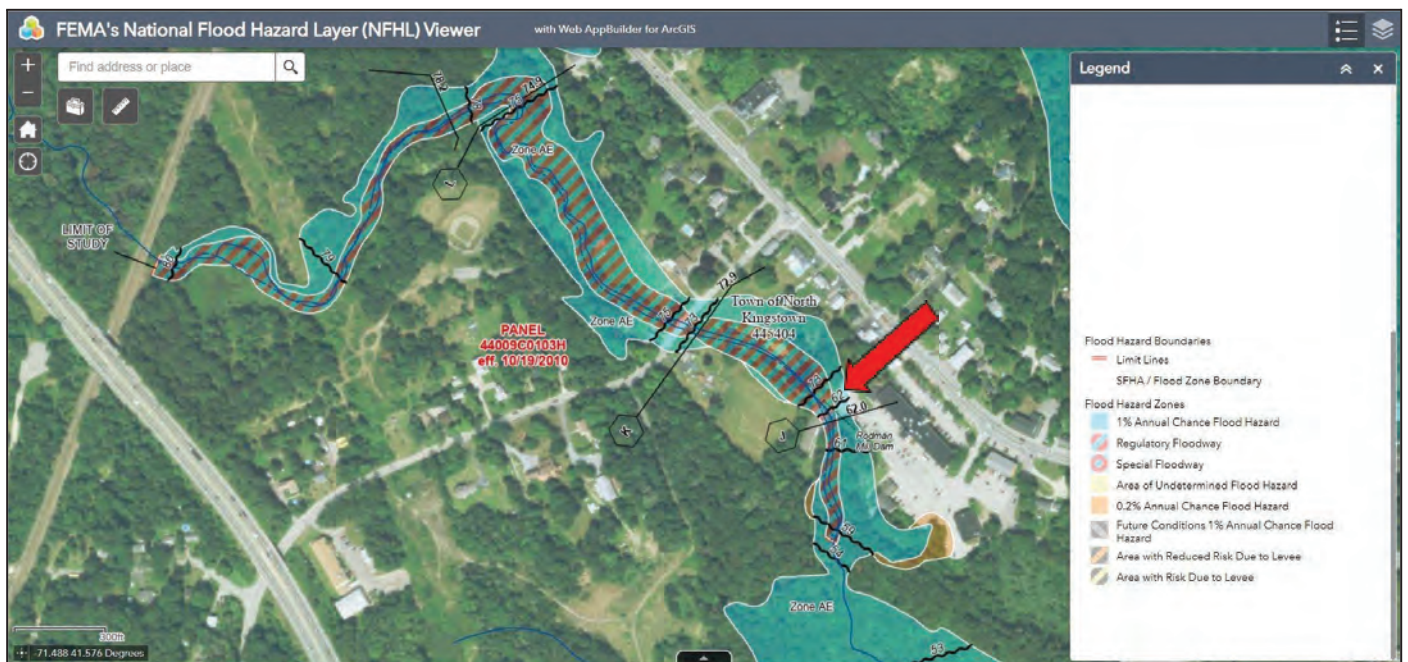
Figure 8: Floodplain and floodways as mapped by Federal Emergency Management Agency (FEMA) of the Annaquatucket River. Red arrow points to the dam. Rodman Mill Dam is categorized as a high hazard dam by RIDEM's Office of Dam Safety.
