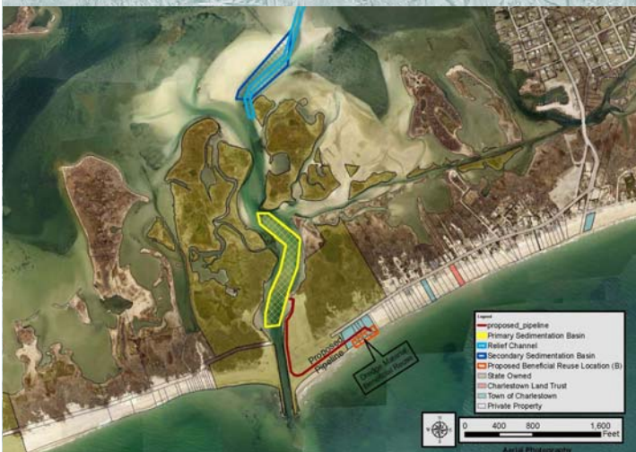
A schematic showing the restoration area, areas to be dredged, and the pipeline location. (Courtesy of Town of Charlestown)
