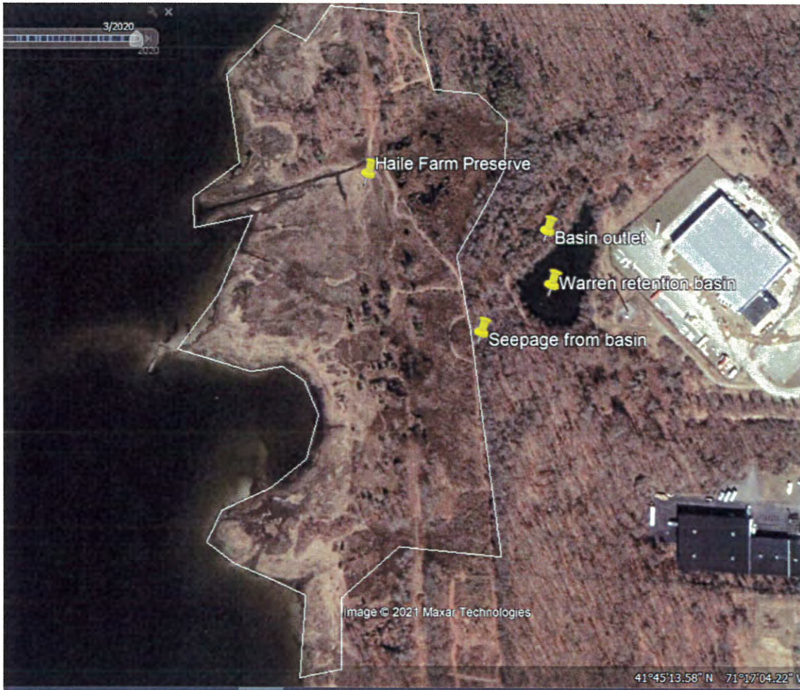
Figure 1: Haile Farm Preserve salt marsh owned by Warren Land Conservation Trust and the retention basin and outlet causing impounded water in the brackish marsh dominated by Phragmites . (2020 Google Earth image)
