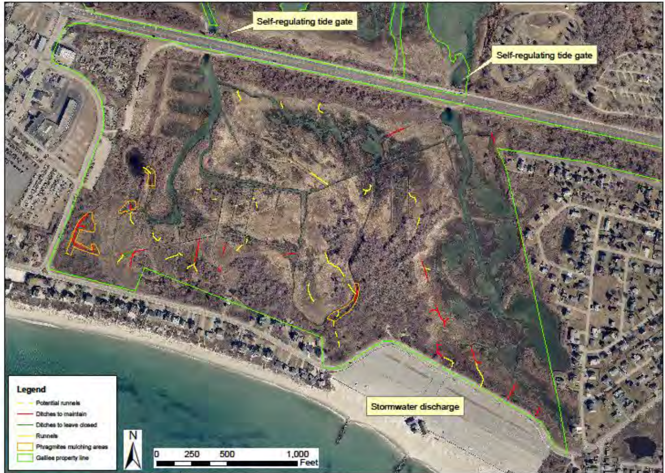
Draft salt marsh restoration plan showing proposed runnels to be installed, drainage features to be maintained and Phragmites to be mulched.
