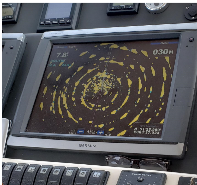
FIGURE 1.3 Photograph of the display of a shipboard radar operated in a U.K. wind farm. SOURCE: Seafreeze, Ltd., included in public comments submitted to the 2019 U.S. Coast Guard Port Access Route Study: The Areas Offshore of Massachusetts and Rhode Island (USCG-2019-0131-0026).
