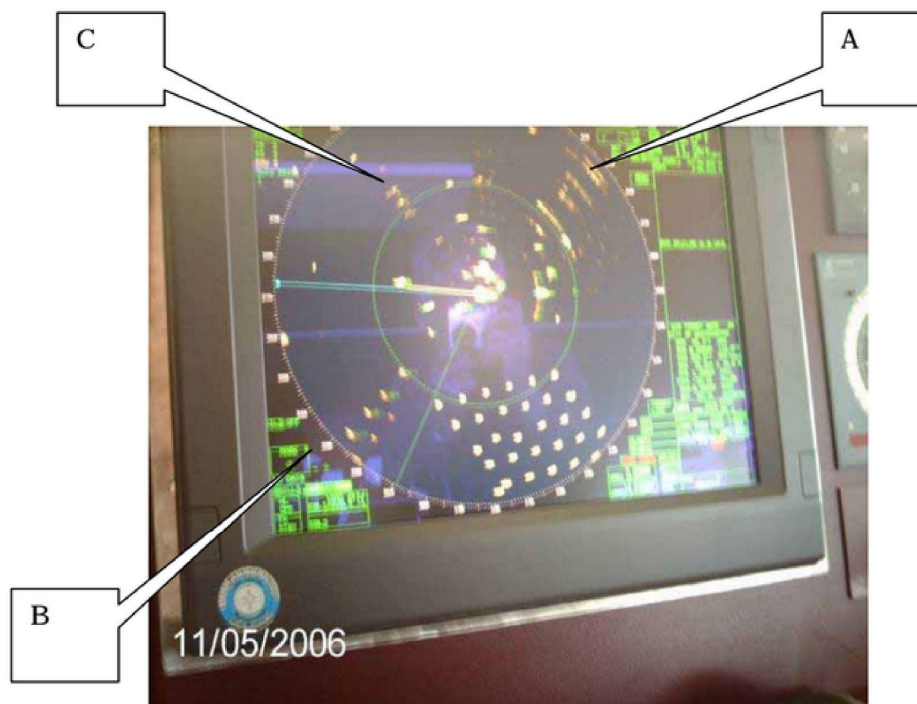
FIGURE 2.10 Illustrative plan position indicator display for magnetron-based radar from the Kentish Flats experiments, where the points A, B, and C highlight the phenomena of multiple target echoes due to wind turbine generator–radar interaction. SOURCE: Marico Marine (2007).
