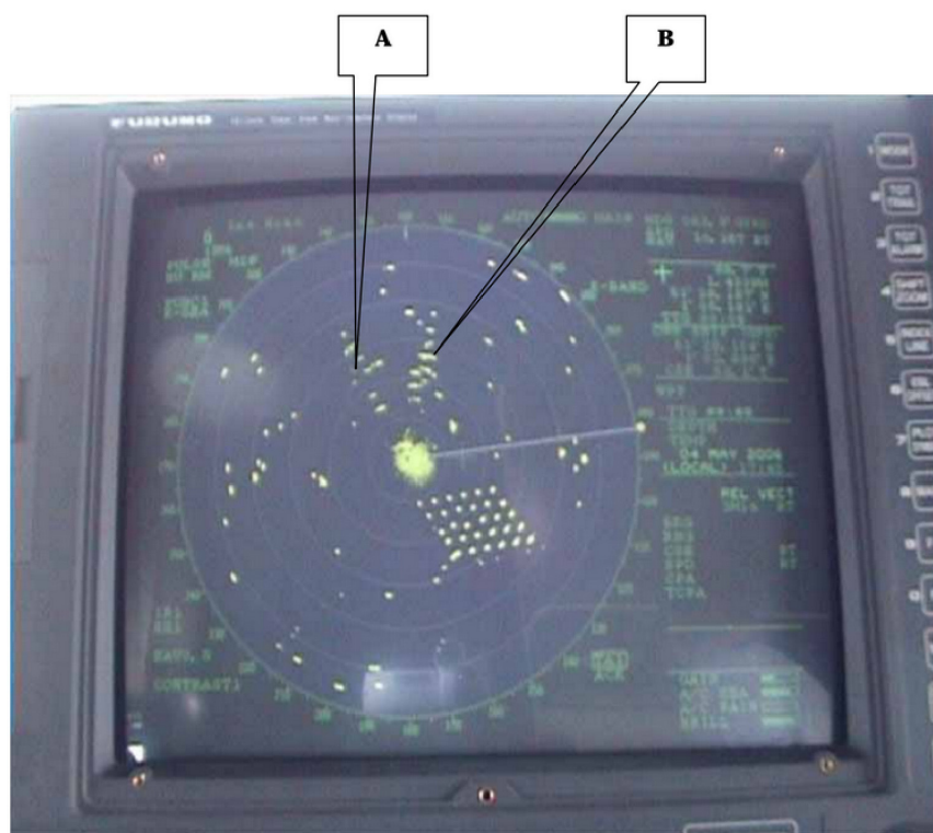
FIGURE 2.13 Multipath example within proximity of wind turbine generators. SOURCE: Marico Marine (2007).
