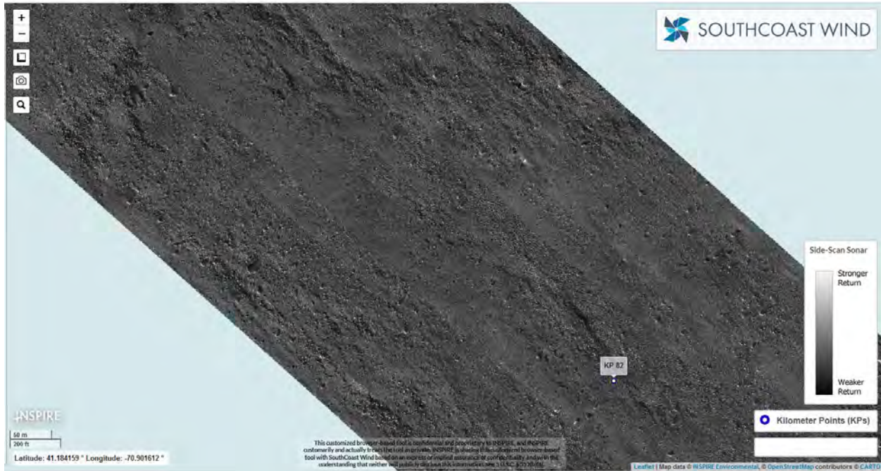
Figure 7: Side-scan sonar mosaic showing the extent of boulders in the vicinity of KP82,
