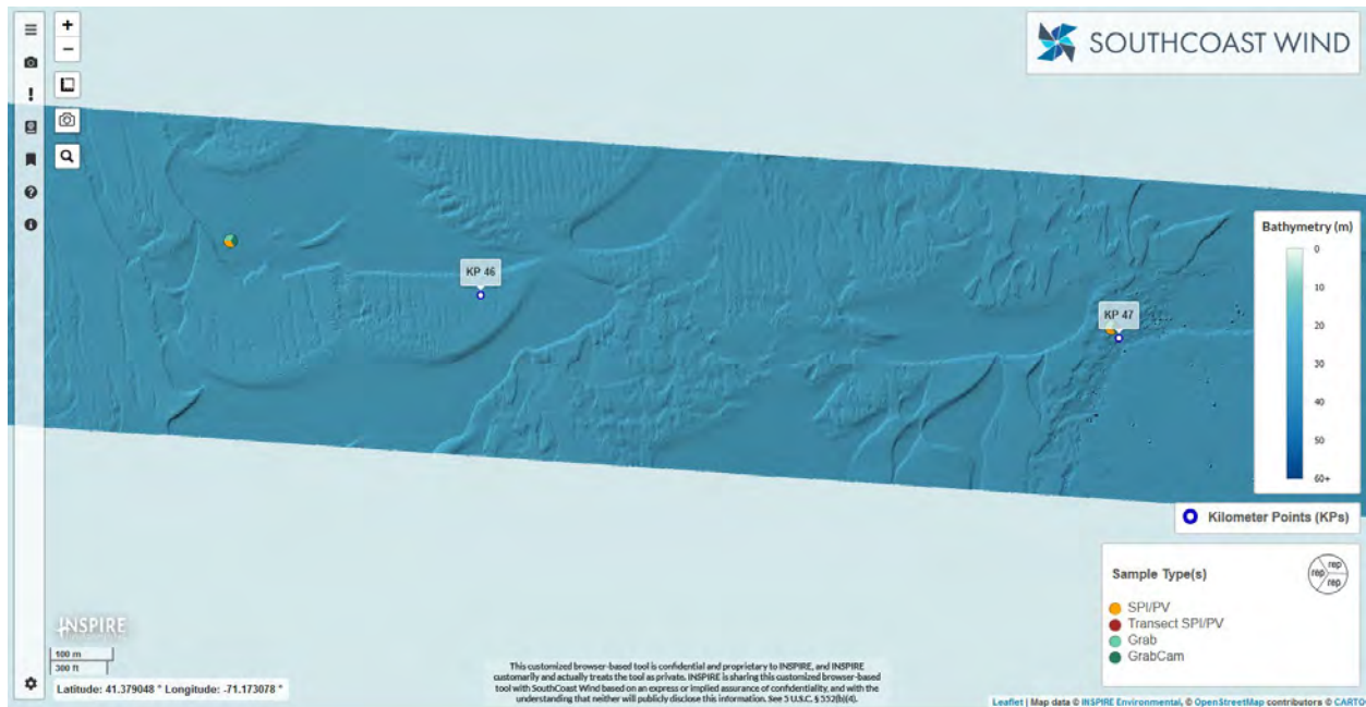
Figure 21: Multi-beam bathymetry around KP46 and KP47 showing examples of the complex sorted bedforms found within the OECC.
