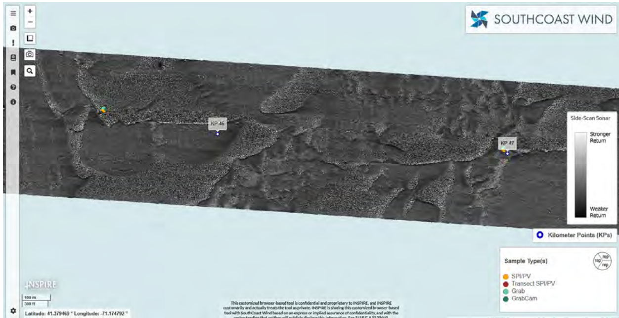
Figure 22: Side-scan sonar mosaic around KP46 and KP47 showing examples of the complex sorted bedforms found within the OECC.
