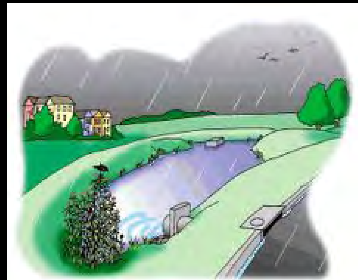
Typical detention pond design
