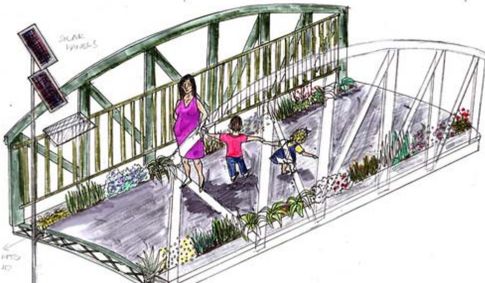
The Green Bridge showing solar panels, informational signage, and vegetated channels with pipes. Rendering by: Rayna Coletta
