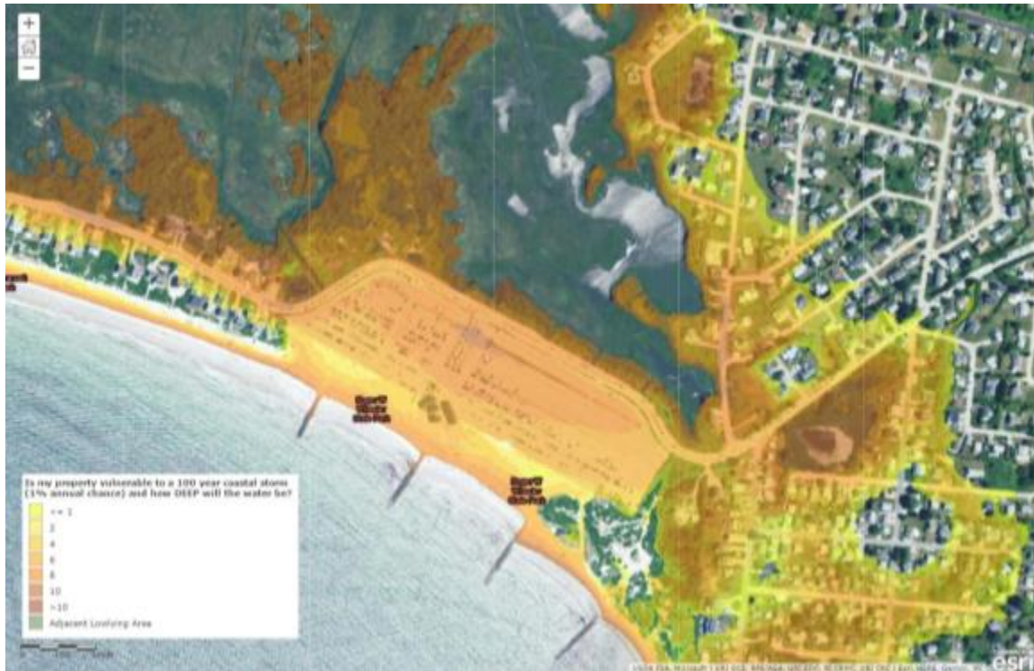
Figure 1. Present-Day Scenario (100-year return period storm surge, no sea level rise) at Roger Wheeler State Park, Narragansett, RI. Colors represent flooding in feet with darker orange representing deeper water. Flooding across the dark section of the beach parking lot in this picture is approximately 7 feet deep. Shades of orange and yellow are used in this figure to represent risk under present day conditions. Map created using STORMTOOLS.
