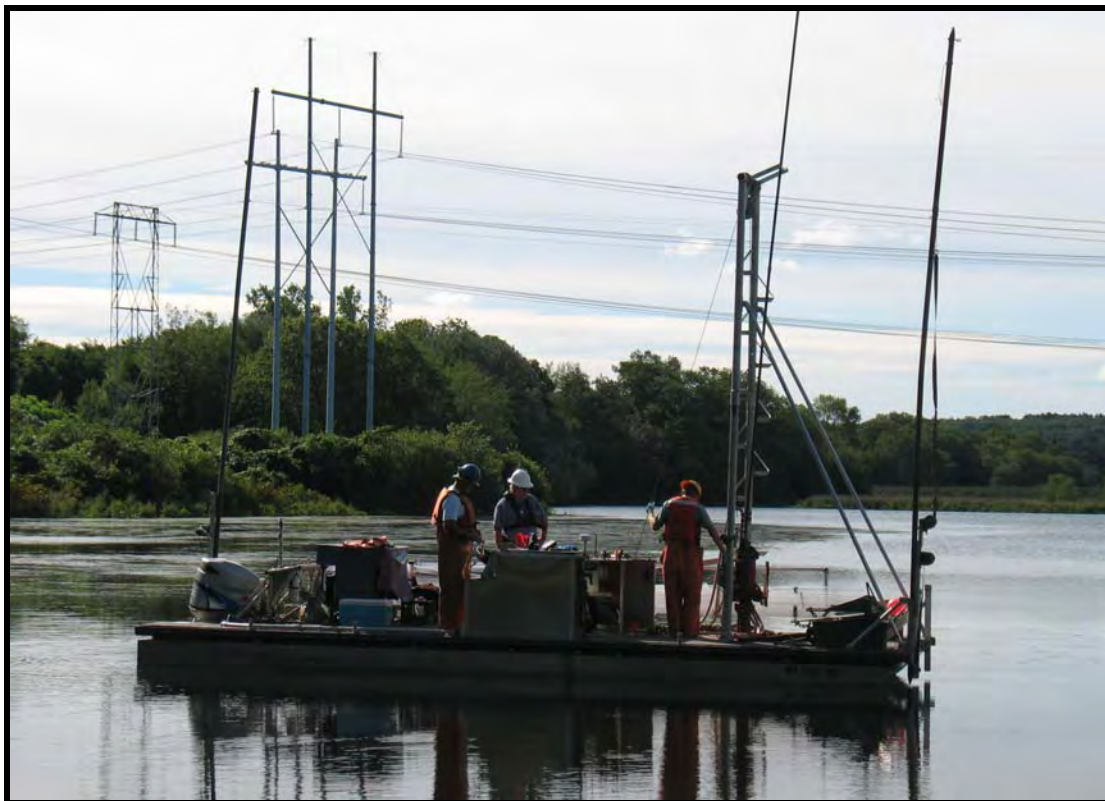
Figure 2 Sediment coring barge equipped with vibracoring rig (in a-frame) and anchoring spuds.
