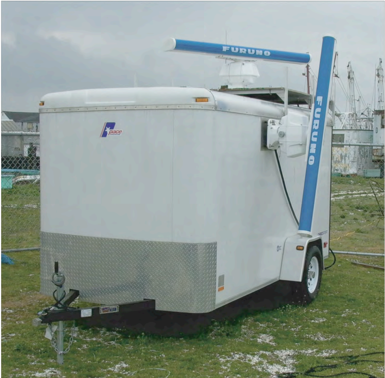
Figure 1. Dual radar system with horizontally and vertically oriented antennas that operate simultaneously. This system allows for data collection on passage (horizontal and vertical), altitude (vertical) and flight direction (horizontal).
