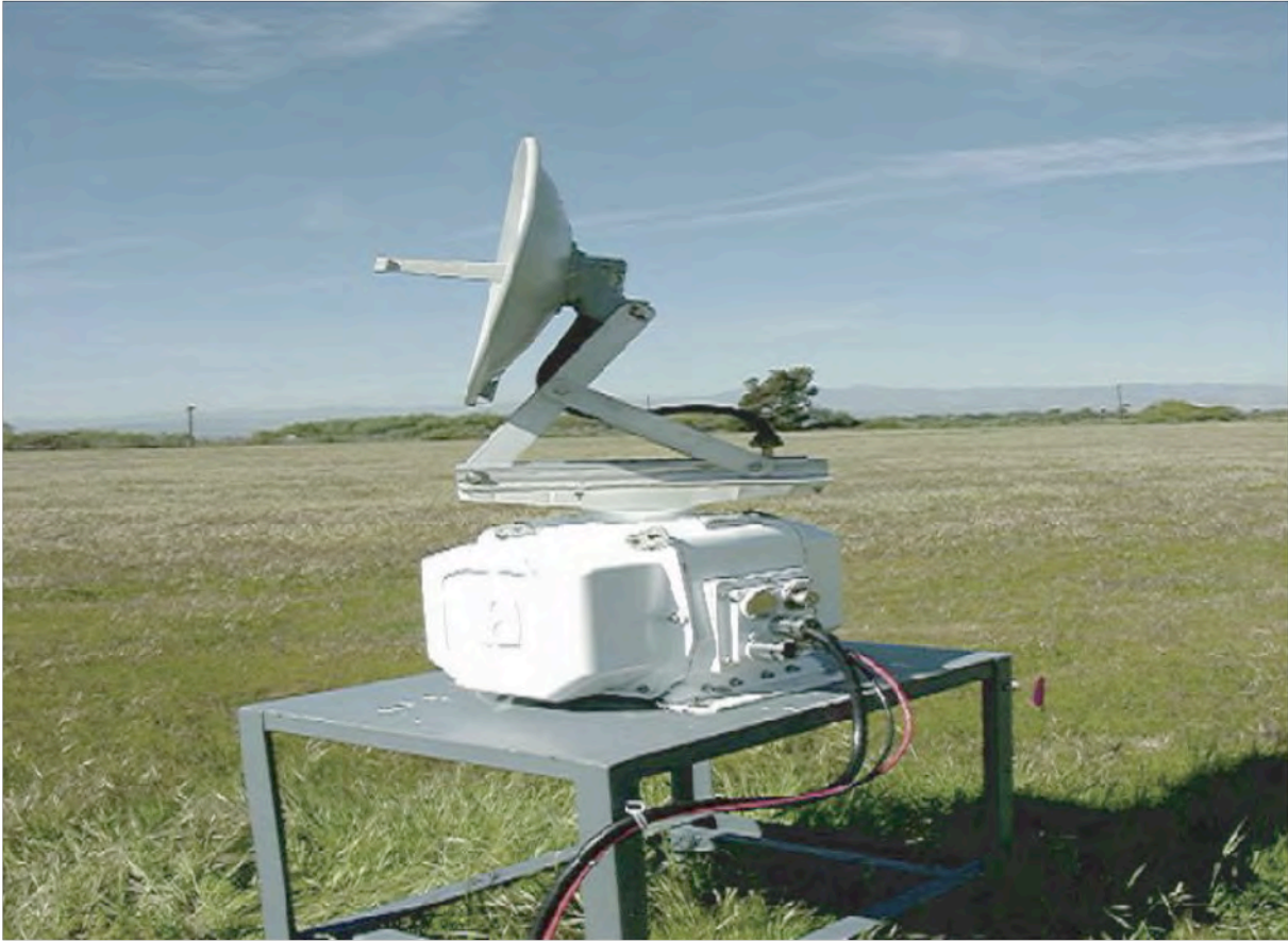
Figure 7. Radar unit with parabollic dish antenna. Custom mounting allow the antenna to be raised or lowered in 2.5° increments above the scanning horizon.
