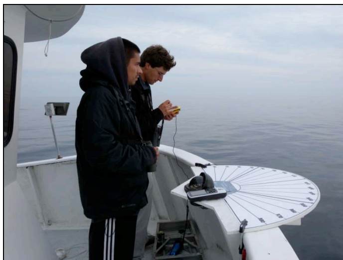
Fig. 25. Ship-based line transect surveys were conducted on a large vessel (>27.5 m), with one primary observer and one observer/recorder. Angle to birds was measured using a large protractor mounted to bridge railing. Note recorder (K. Winiarski) taking observations on a PDA, while primary observer (B. Harris) is actively searching for birds with both naked eye and binoculars.
