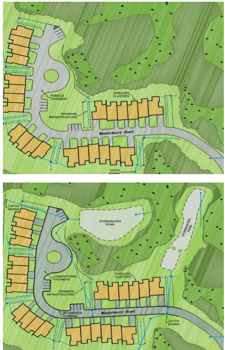
Figure 1. Comparison of two designs, LID design (above) and conventional (below), for Boulder Hills, Pelham, NH
