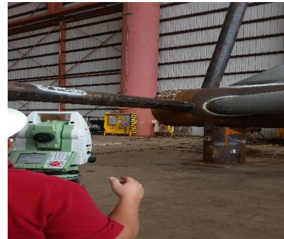
Dimensional inspector surveying deck legs A1 and A2 for site 1
