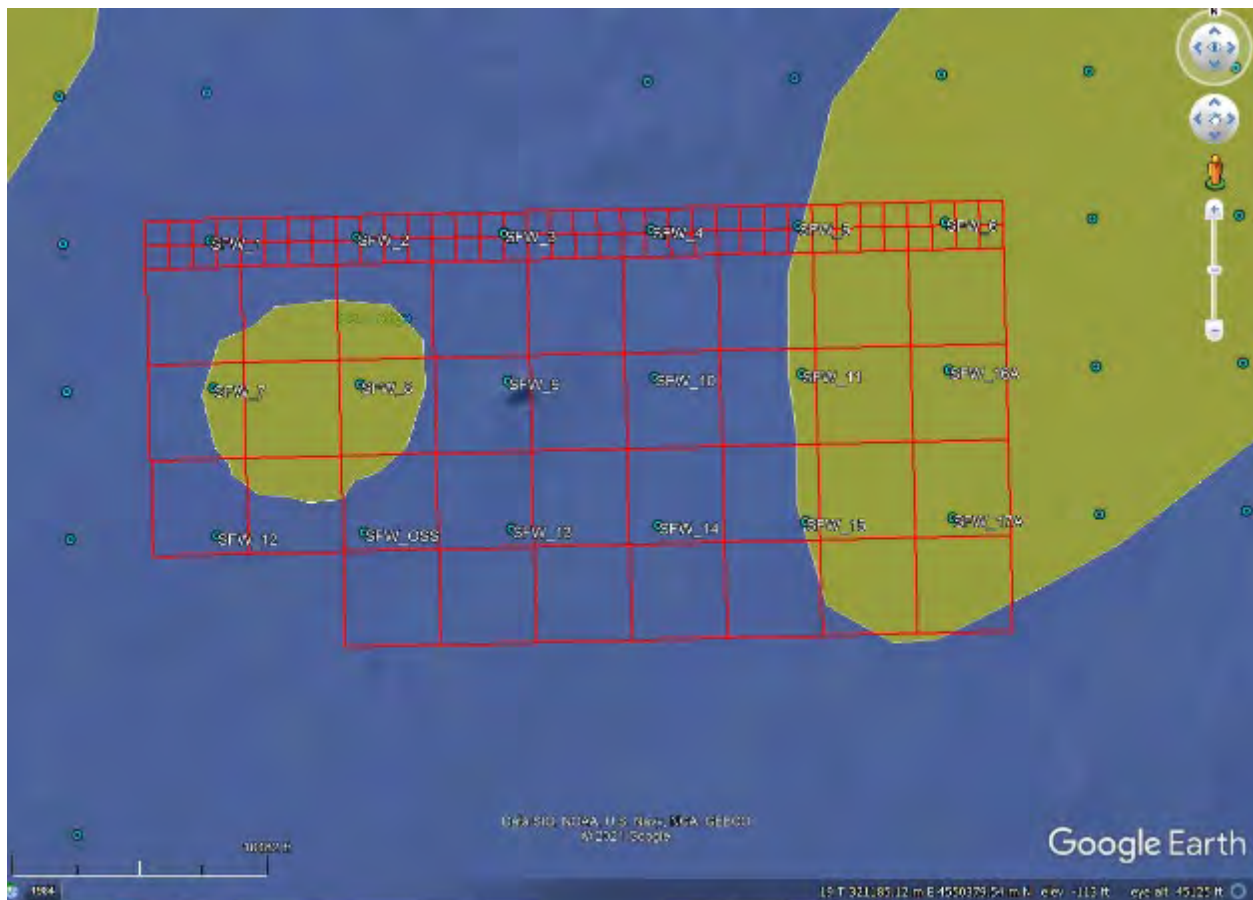
Figure 17. South Fork Wind turbine locations (based on wind industry 1 x 1 uniform grid layout provided by Ørsted on 1/28/20) within the OCS-A 0517 lease area represented by red lines. The yellow shaded polygon areas are glacial moraine and meet the requisite criteria as Areas of Particular Concern (APC) as identified by the CRMC in the enforceable policies.
