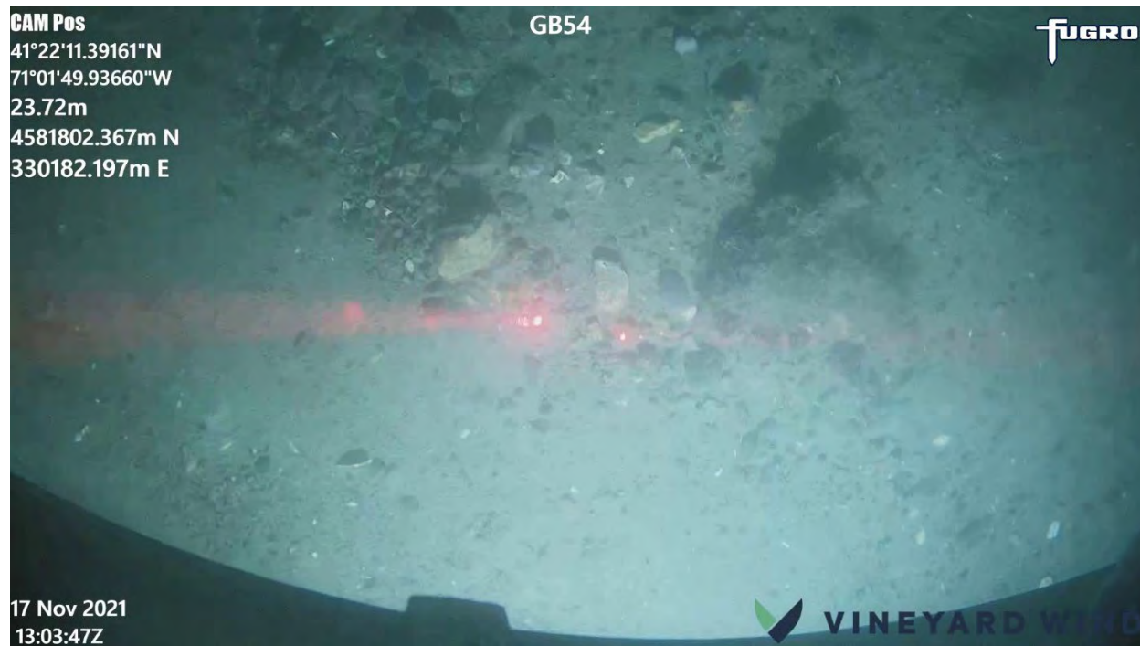
Figure 16: Plan view image of the seafloor at station GB-54 located southwest of Cuttyhunk along a portion of Browns Ledge. The sediment here is mapped as sandy gravel. See figure 11 for the location of the sample.
