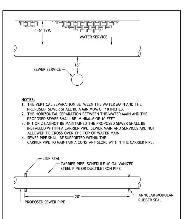
SEWER/WATER SEPARATION DETAIL
