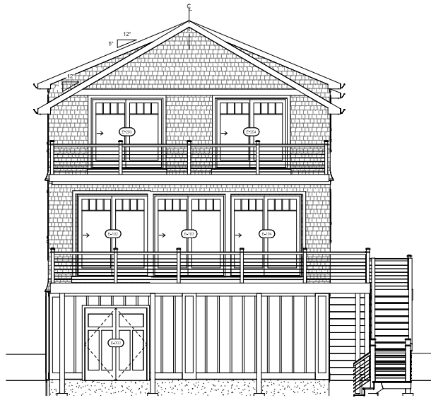
3 EXTERIOR - REAR ELEVATION - EAST 1/4" = 1'-0"
