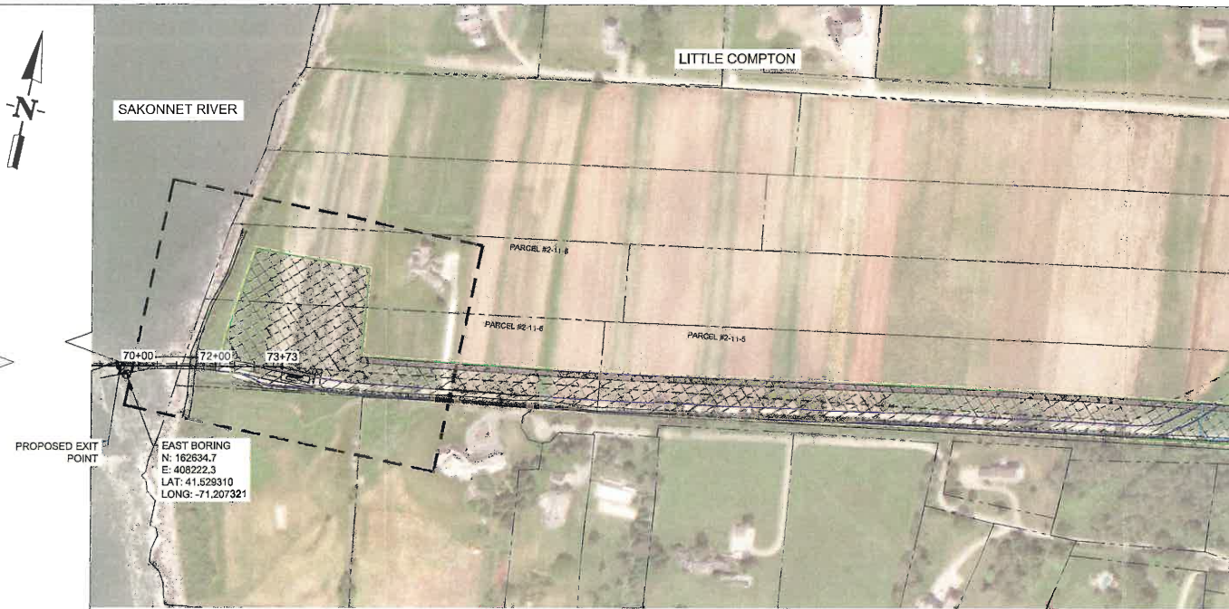
2 HDD SAKONNET EAST CROSSING PLAN 1"=200'-0"
