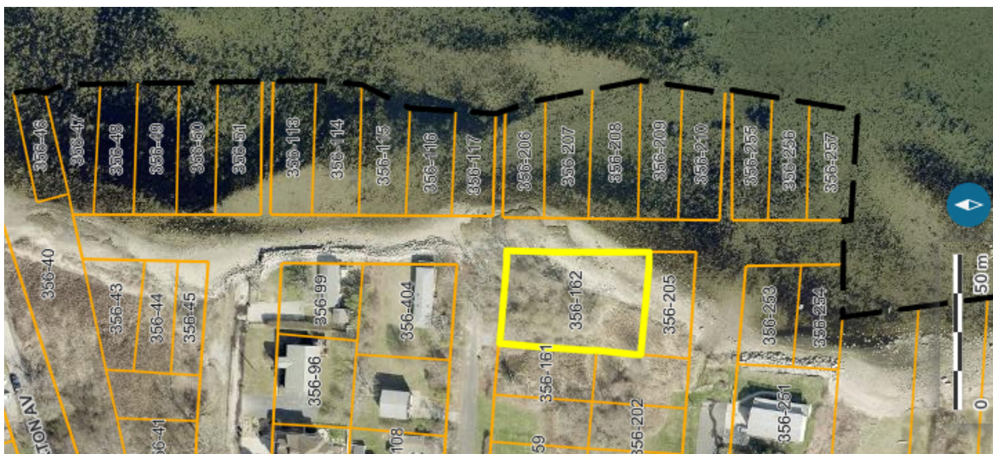
Figure 8: City of Warwick, RI axisgis.com plat map showing the now abandoned Seashore Rd. running north/south (left/right on image) and 19 City of Warwick owned parcels, now in Narragansett Bay, between Samuel Gorton Ave to the north (left) and Grove Ave. to the south (right).
