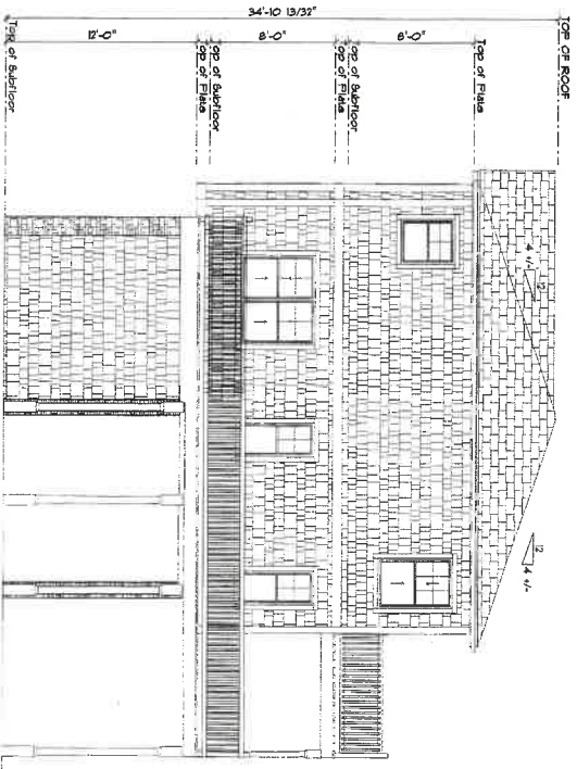
RIGHT SIDE ELEVATION 1/4"=1'-0"
