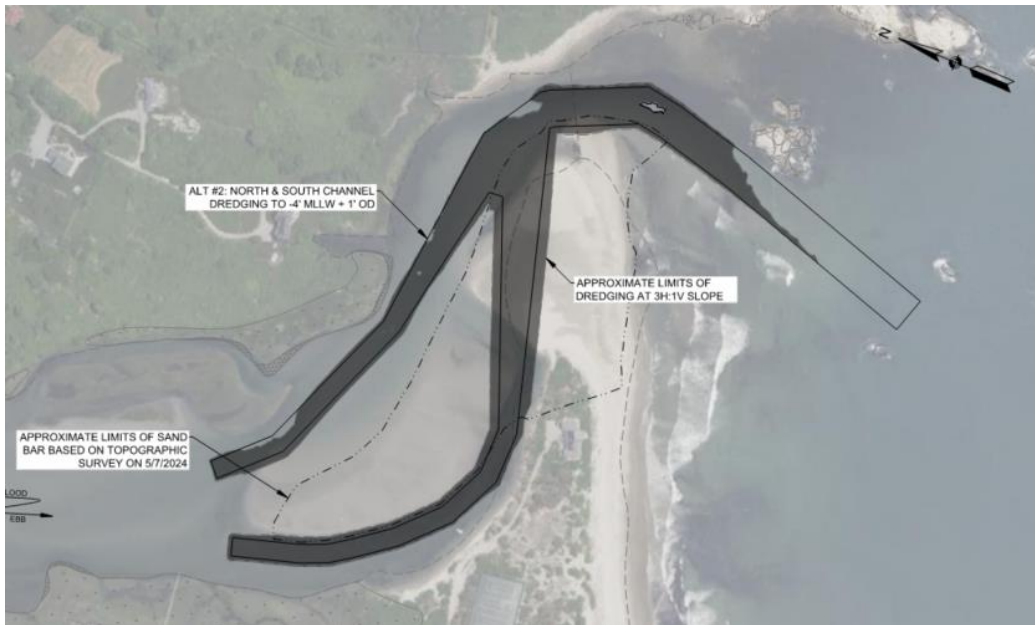
Figure 3-2: The Narrows Channels Dredging
