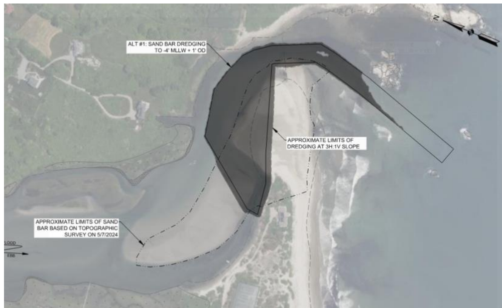
Figure 3-1: Narrow River Entrance Dredging
