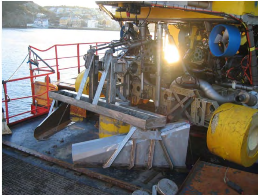
Figure 18. Capjet Backfill Plow
