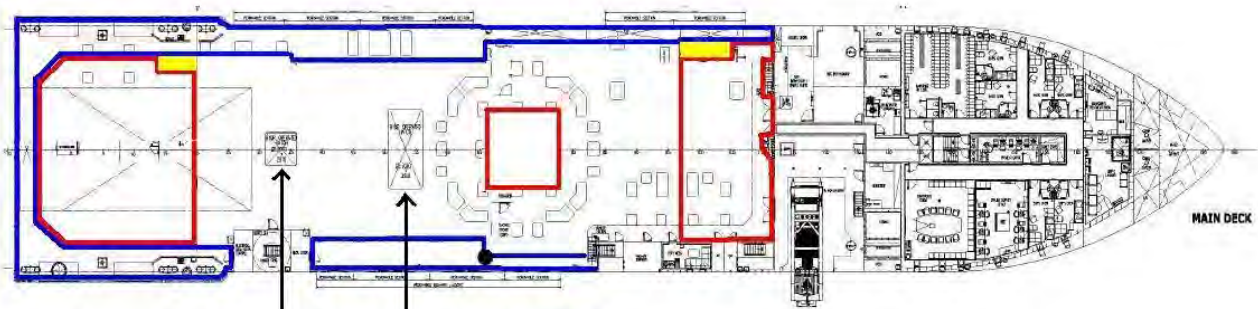
On main deck there are 2 hatches that cannot be welded on
