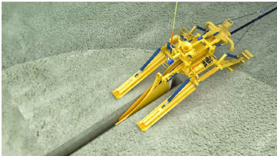
Figure 15. Cable Secured into the Jet Plow
