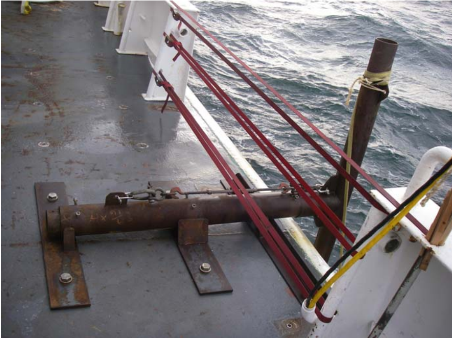
Figure 5: Picture showing pole mounting system secured to ship's deck.
