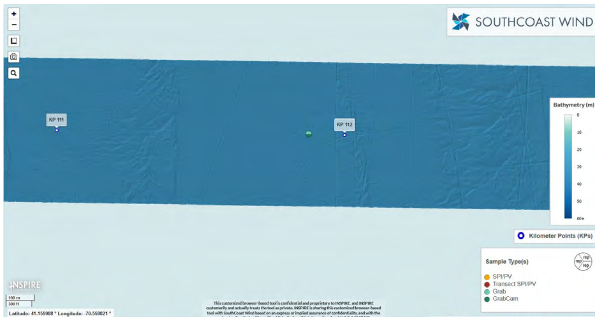
Figure 23: Multi-beam bathymetry showing examples of hydraulic dredge scars around KP111 and KP112.
