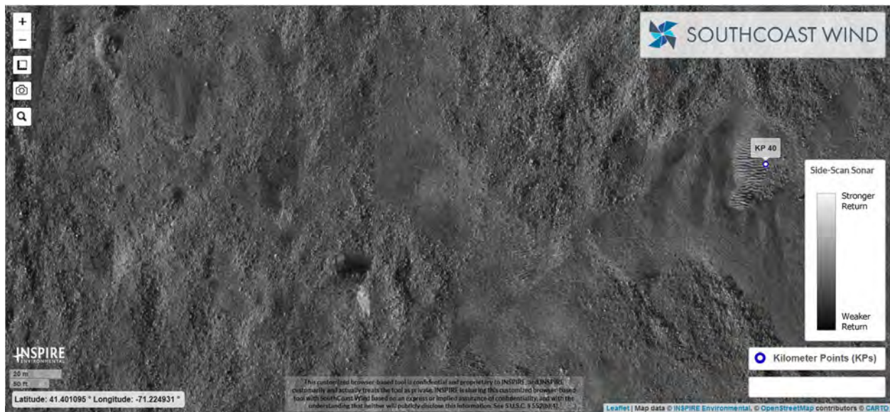
Figure 15: Side-scan sonar mosaic near kilometer post 40 showing widespread cobbles and boulders.
